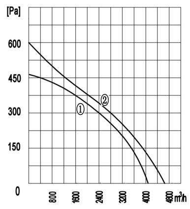
Curve 1: 50HZ Curve 2: 60HZ
